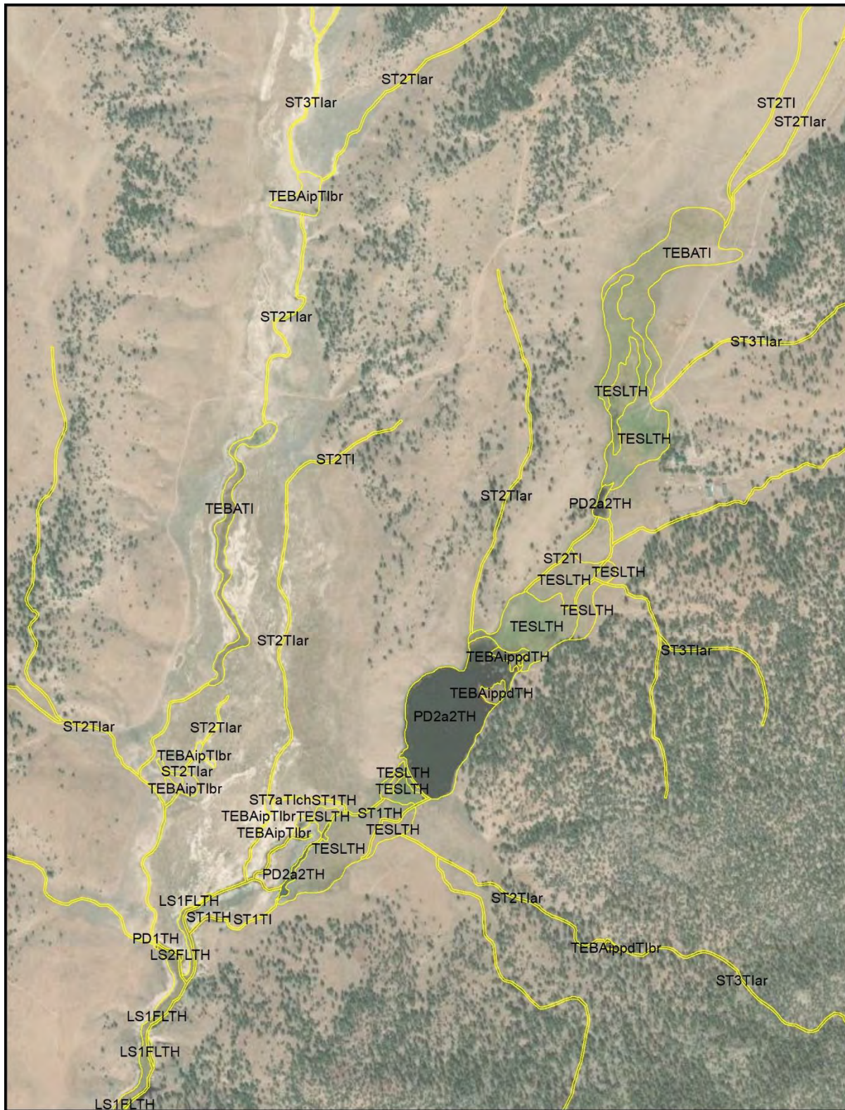
Figure 17. Aerial photography over Catron County, along Centerfire Creek, viewed at a scale of 1:15,000. After completion of the wetland delineation, the image interpreter has assigned LLWW attributes to each wetland.
