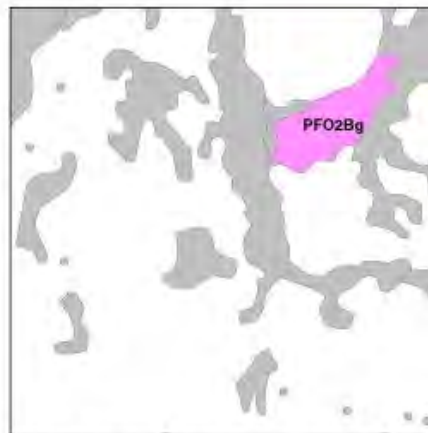
d.) The organic soils modifier 'g' is added to the code of the wetland polygon that intersects the organic soils polygon.
