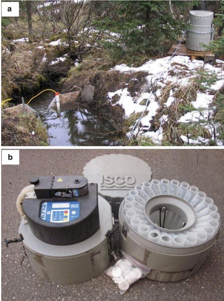
Fig. 3.32 Automated sampler for collecting stream water samples at a prescribed time interval. (a) A field sampler with the sample intake in a pool above a V-notch weir. (b) The same sampler showing the control unit and 24 sample bottles inside the sampler body (Photos by Masaki Hayashi)
