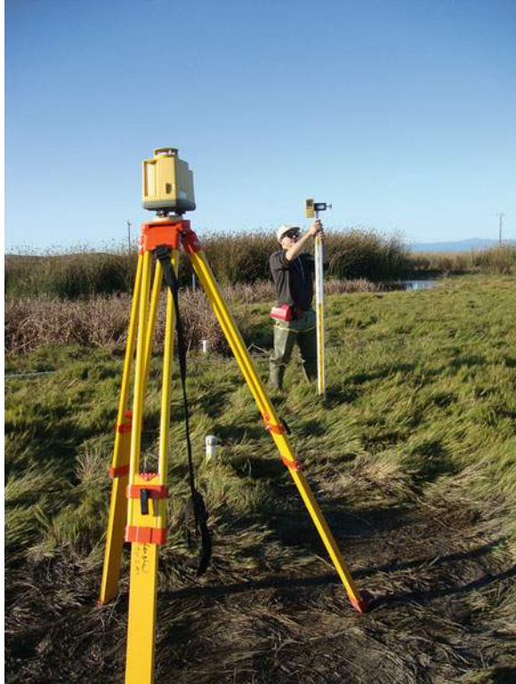
Fig. 2.11 An example of rotating laser equipment, which can be used by a single person
