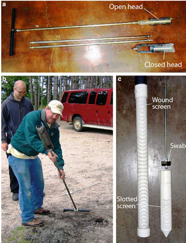
Fig. 3.42 Hand auger for removing sediment prior to installation of a water-table monitoring well. (a) Auger head, rod, and handle with two rod extensions and an additional auger head; (b) Augering a hole with the bucket inverted for removal of sediment; (c) PVC wound well screen, PVC slotted well screen, and well-screen swab. Note the two different types of fittings at the end of the well screen (standard PVC cap and cone-shaped PVC point). If the slotted screen is inverted and the cap is attached to the opposite end, the non-slotted interval becomes the sump
