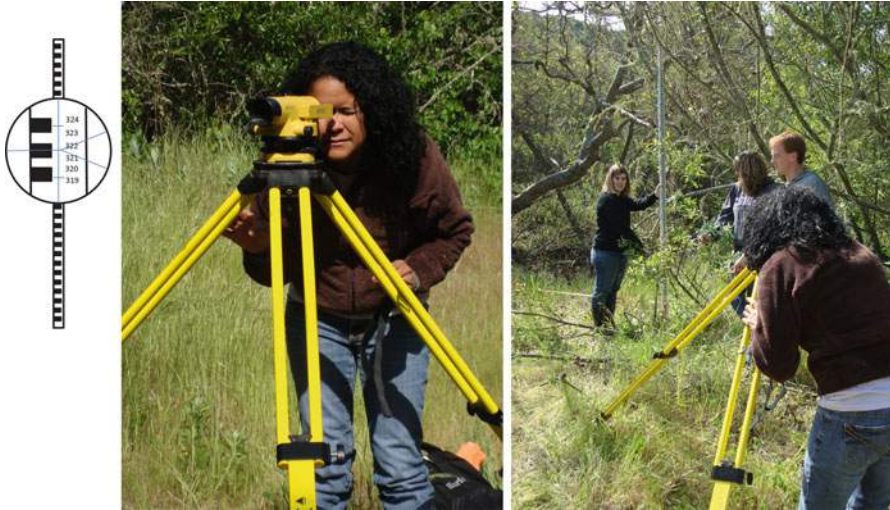
Fig. 2.10 Autolevel surveys are a series of “shots” in which a rod reading is recorded. The colored blocks are 0.01 m tall, and every 0.01 m has a number. This shot indicates that the ground elevation is 3.215 m below the optical center or instrument height (HI) of the scope
