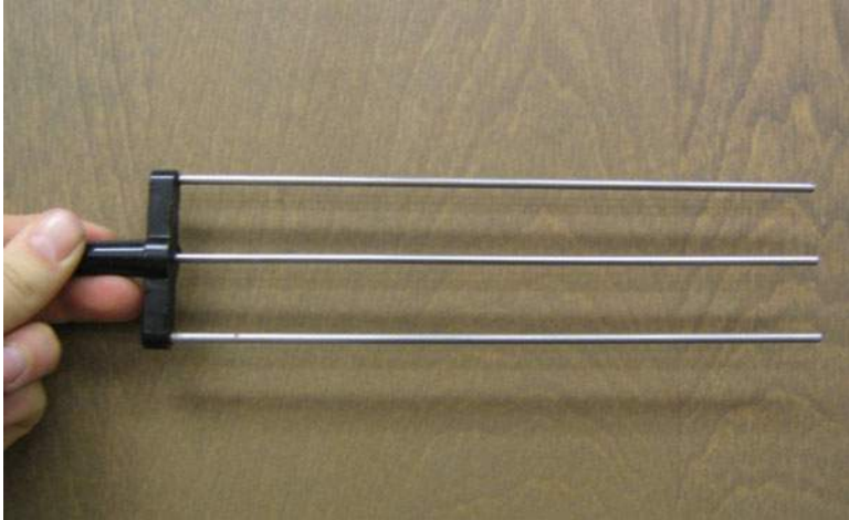
Fig. 3.29 Example of a parallel-rod wave guide for time domain reflectometry (TDR)
