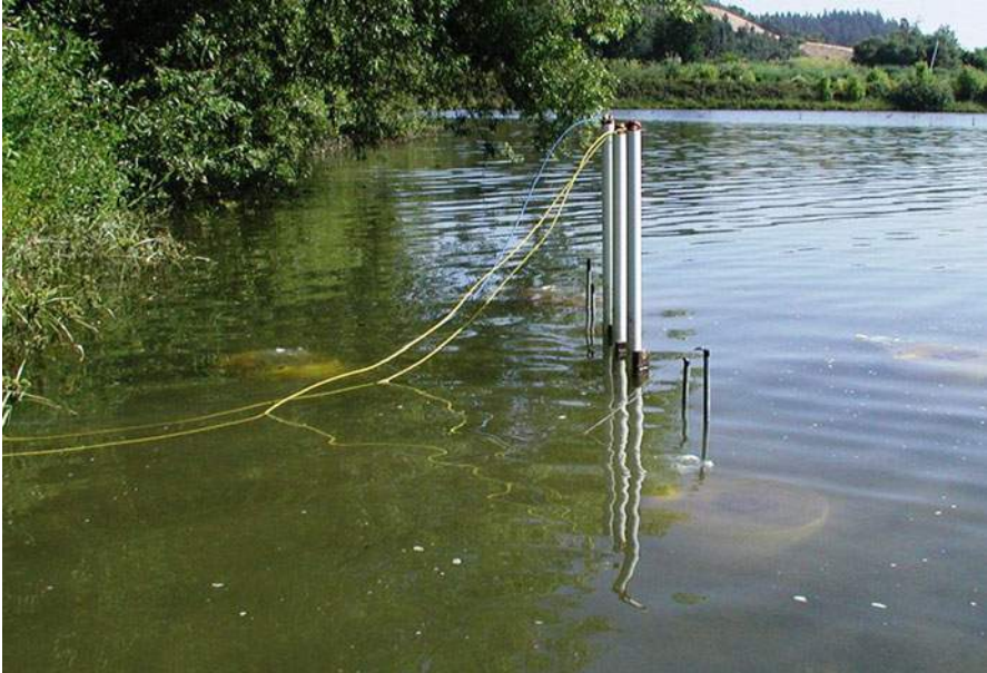
Fig. 3.46 Nest of piezometers installed at different depths beneath the wetland bed with pressure transducers and temperature sensors installed in five of the seven wells. All sensors are connected to a digital datalogger positioned on shore to the left of the photo. Note also the four seepage meters, with bags attached directly to the tops of the seepage cylinders, installed near the wells. Attaching the bag directly to the seepage cylinder is sometimes acceptable where wind and currents are minimal
