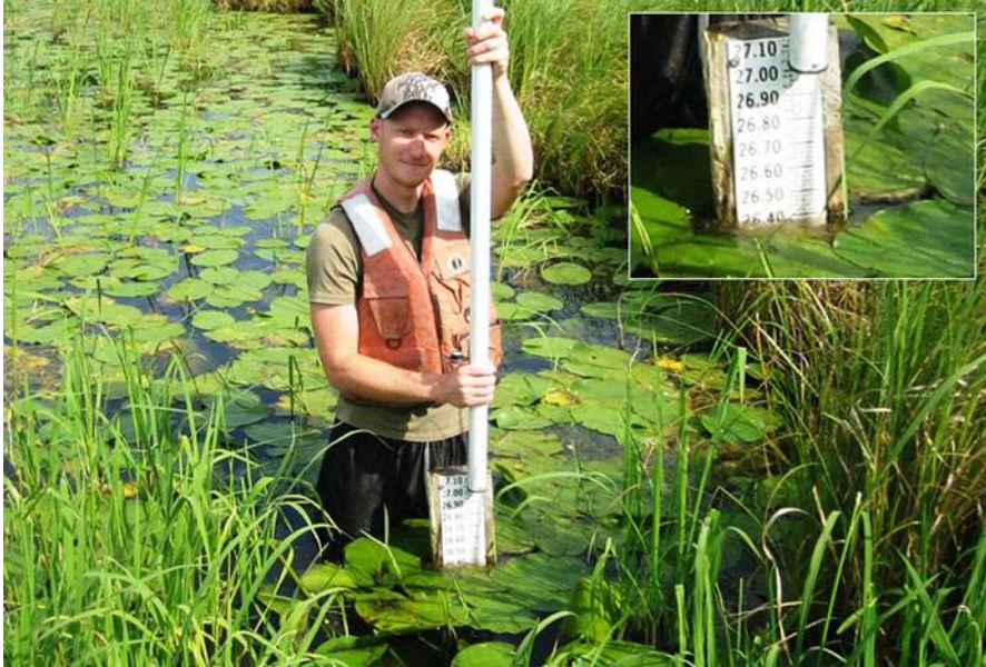
Fig. 3.2 Surveying a wetland staff gage to a local datum. Rod is held on a screw projecting from the plank on which the staff plate is mounted. Water-level is at 26.38
