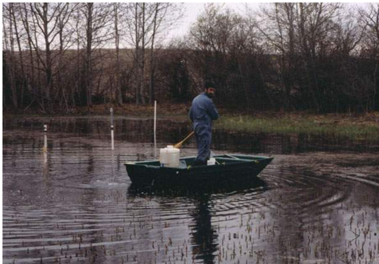
Fig. 3.33 Application of bromide tracer in a prairie wetland (Parsons et al. 2004). To ensure even distribution of tracer, the tracer solution was slowly released to the wetland from a boat moving around the wetland (Photo printed with kind permission of © David Parsons 2012. All rights reserved)
