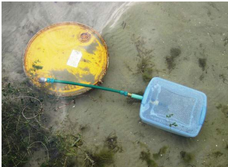
Fig. 3.25 Half-barrel seepage meter with seepage bag located inside a bag shelter for protection from currents and waves (Photo by Donald Rosenberry)
