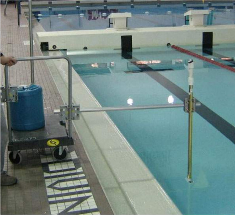
Fig. 3.15 Calibration of a horizontal-axis current meter in a swimming pool. The meter is attached to a cart that is pushed at a constant velocity (Photo by Masaki Hayashi)
