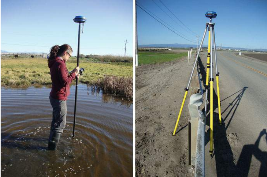
Fig. 2.13 An example of real-time, kinetic GPS (RTK GPS) equipment. The base ( right ) and rover ( left ) can communicate with each other up to several kilometers with radio signal booster. RTK GPS is efficient and requires only one operator
