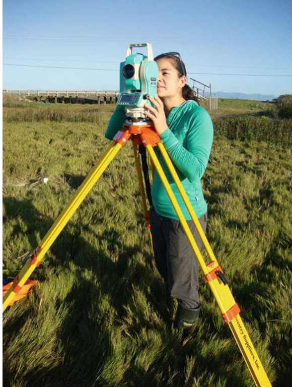
Fig. 2.12 An example of total station equipment, which can be used to rapidly capture precise X, Y, and Z points
