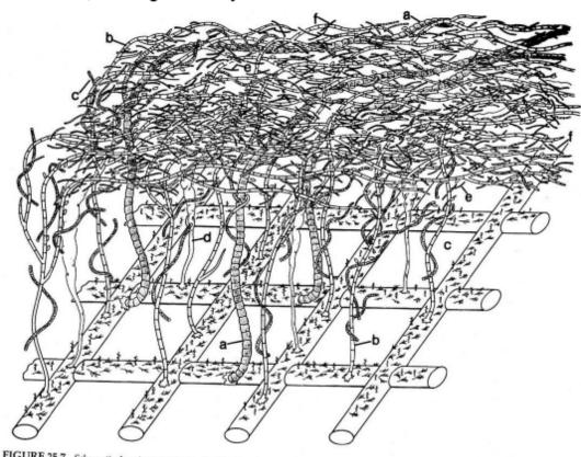
This technology contrasts with most algal growth systems that utilize suspended algae instead of attached algae. One advantage of the ATS is that attached algae are easier to harvest than suspended algae.
