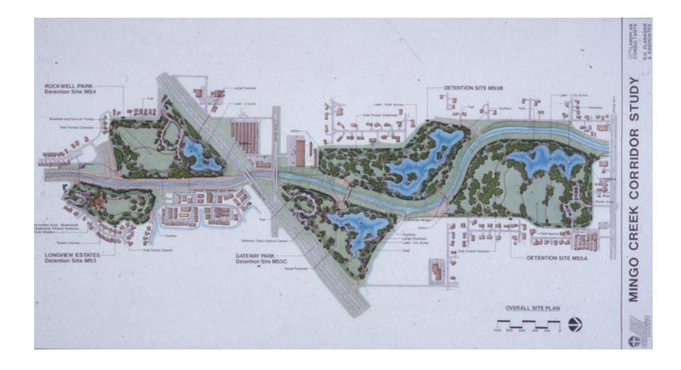
City of Tulsa/Corps of Engineers' Plan for Stormwater Detention Ponds along Mingo Creek
