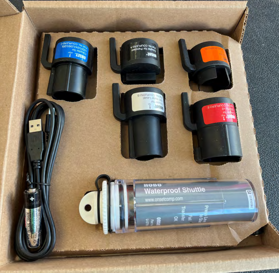
Hobo Waterproof Shuttle to set and read Hobo Data Loggers
